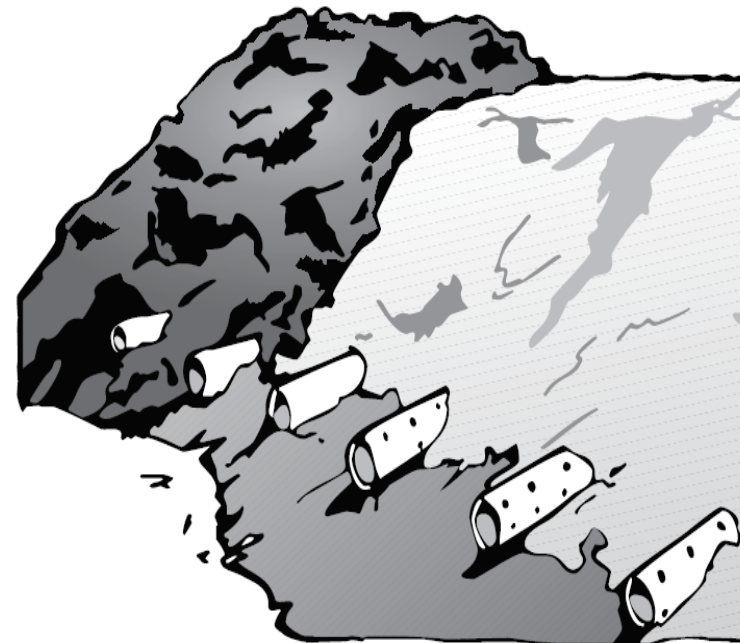
Aerated static pile with perforated PVC pipes.
